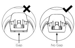
**5.3** Push the lever down to secure it to the arm assembly
