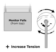
**7.4** If the monitor springs upwards from the bottom position, decrease the arm tension by rotating the screw anti-clockwise.
