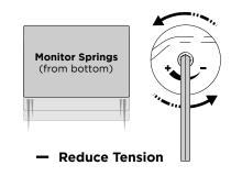
**7.5** If the monitor floats or hovers in all positions the arm tension is balanced and does not require further adjustment.
