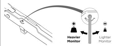
**7.3** If the monitor sags or falls down, increase the arm tension by rotating the screw clockwise.
