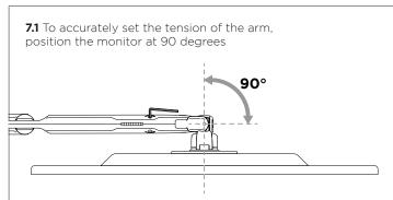
**7.2** Use the allen key to adjust the arm tension to the weight of the monitor. Follow steps **7.3** to **7.5** to set the tension.
